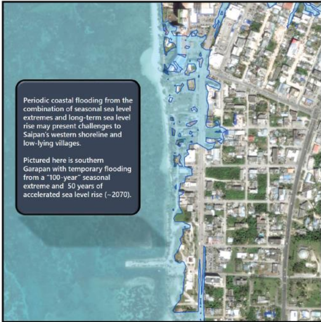
Fig. 17. Satellite image of southern Garapan with an overlay showing the extent of possible future coastal flooding from a combination of an extreme sea level event and long-term sea level rise. The map illustrates the scale of potential flooding, not the exact location, and does not account for erosion, subsidence, or future construction. Water levels are shown as they would appear in 2070 with sea level rise under a high warming ("business-as-usual") scenario and with a "100-year" high seasonal sea level event. Planning for structures with an expected 50-year or greater lifespan might consider such a scenario. Source: Figure courtesy of Robble Greene and CNMI BECQ.
